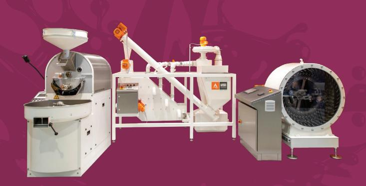
For manufacturing of fine chocolate mass using raw cocoa beans incorporating roasting, winnowing, liquor pre-grinding, chocolate refining & conching
